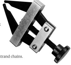
Although primarily for Simplex chains, these pullers can also be used for multistrand chains.
